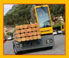
Over 8 hours continuous run time, panoramic cabin, load sensing, joystick control, full road-legal LED lighting and precise mast control makes this durable machine one of the most productive and energy-efficient ever made.
