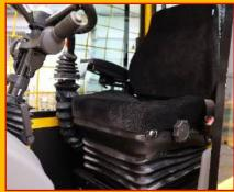
A completely re-engineered operator cabin is at the heart of the EXL, designed to transform comfort and usability. 20% larger than the ELX model, with an 800mm width, 200mm added in length, and a 100mm increase in height, it allows a larger ergonomic seat, increased legroom and arm movement, and an entirely new dashboard layout for optimal control and visibility.
